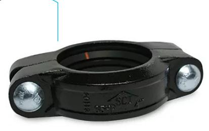
Figure 65HP–ES couplings with End Shield gaskets are designed for use in high pressure piping systems with working pressure ratings up to 2,500 psi.\*
